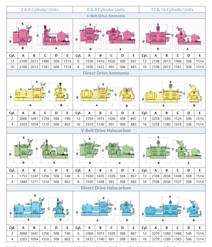
General Dimensions – The dimensions shown above are approximate, and should not be used for construction. Vilter issues certified prints for construction purposes. These dimensions are provided in millimeters. Space needed to remove flywheel 178mm. Space needed to remove crankshaft, from wall to centerline of compressor 1067mm for 2-8 cylinder models, and 2134mm for 12-16 cylinder models.
